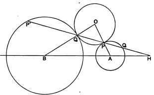
Let a circle be drawn touching two given circles in the points P and Q. Then, if O be its centre, and A and B the centres of the given circles, it is evident that AP, BQ' are equally inclined to PQ'. Therefore, if PQ' cut the given circles in Q and P', AQ and BQ' are parallel. Therefore PQ must pass through H, one of the homothetic centres of the given circles.
